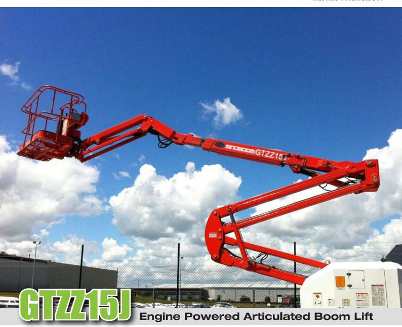
**EASY-TO-USE CONTROLS** - both ground and platform feature a workstation making it quick and easy to get right to work. **ROUGH TERRAIN PERFORMANCE** - oscillating axle and 4-wheel drive improves rough terrain capabilities and drive performance. **OUTSTANDING PROTECTION** - steel covers adopted to protect the inside parts better and easy to open. **GREATER ACCESS** - the standard configured jib gives you even easier access to hard-to-reach places.
