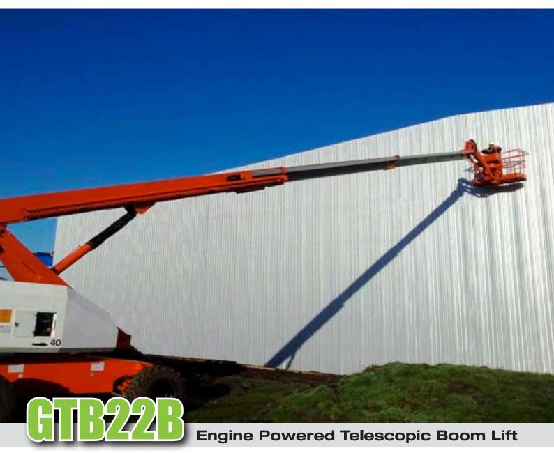
ROUGH TERRAIN PERFORMANCE - Oscillating axle and 4-wheel drive improves rough terrain capabilities and drive performance.
